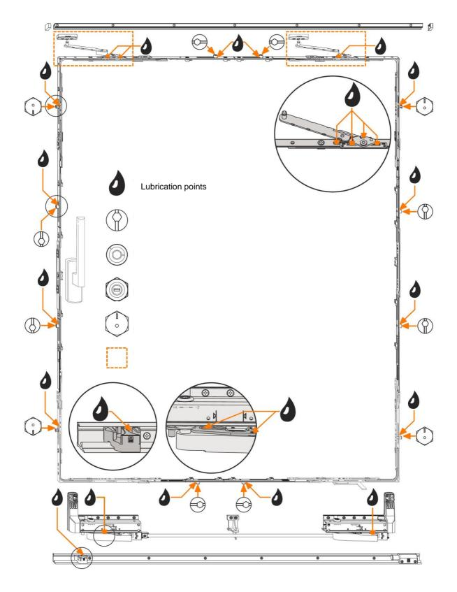
Fig. 20 Lubrication of fittings in tilt and slide sash (lubricants without acid and resin spray are recommended)
