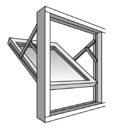
Top Guided reversible fittings allow to turn the sash by 170 o and include a mechanism which prevents opening "A". which works in 2 stages. The first stage enables rotation up to 10 o.
