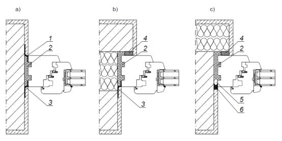
Fig. 9. Window sealing depending on the wall structure
