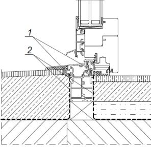
Fig. 14. Sealing of the balcony door with aluminium threshold
