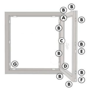
Fig.16. Window adjustment points
