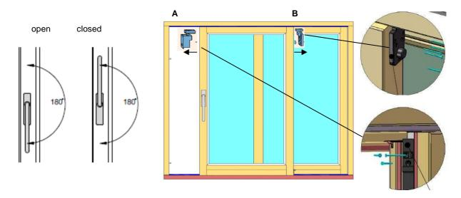
Fig. 21 Removing the sashes
