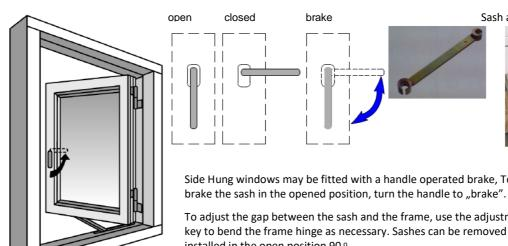
Side Hung windows may be fitted with a handle operated brake, To
