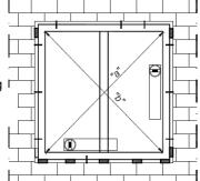
Fig. 4. Checking the window frame setting in the wall opening
