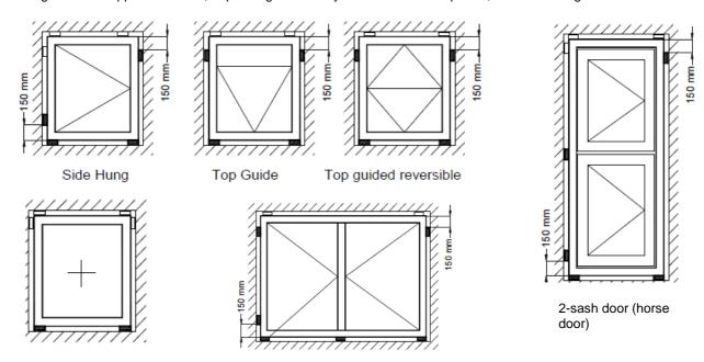
Fig. 5. Basic arrangement of support points for EURO windows
