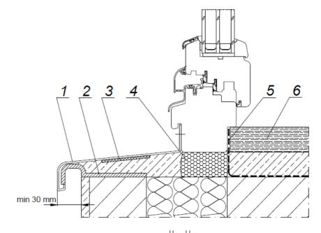
Fig. 10. Example of fitting exterior and interior window sill
