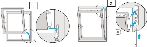
Fig. 15. Installing the sashes
