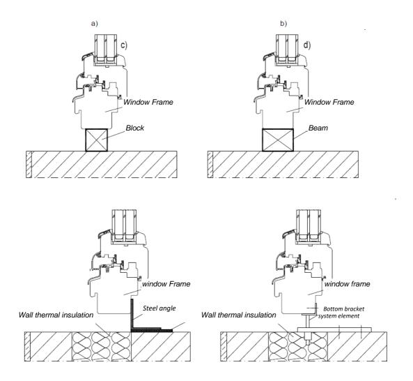
Fig.2 Methods of supporting the window frame threshold
