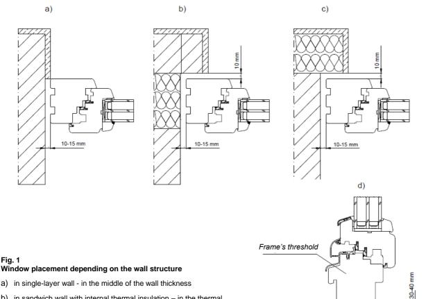
Fig. 1 Window placement depending on the wall structure
