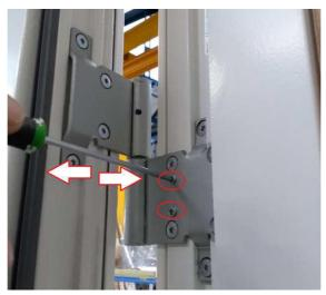
c) Use key/screwdriver with Torx 20, please tighten all screws loosen before marked with letter A
