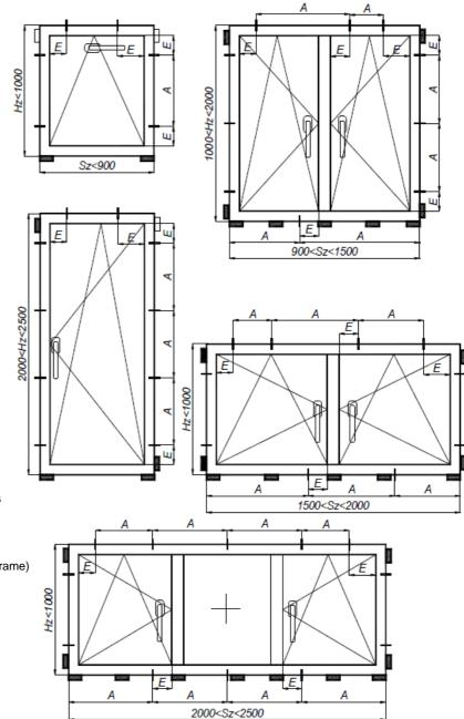
Fig. 3 Window support and fixing points
