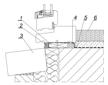
Fig. 12. Example of window threshold sealing in wall with brick outside sill
