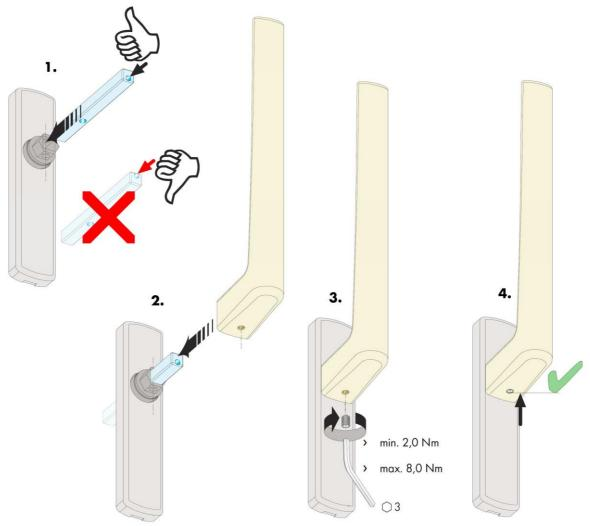
Fig.22 Installing handles in HS lift and slide door
